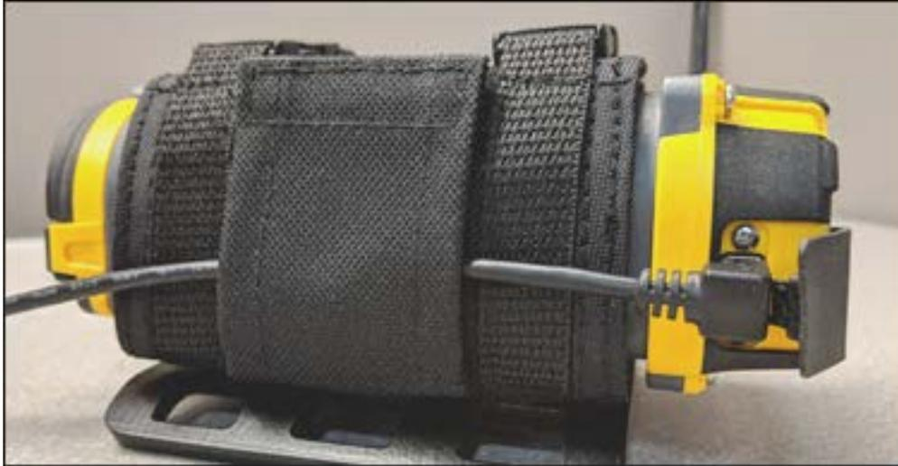
5. Attach the power cable and antenna cable to their connectors on the charge base.
